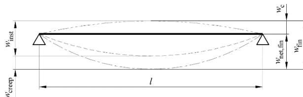
The limiting values for deflections of beams are assumed as shown in the following table.
