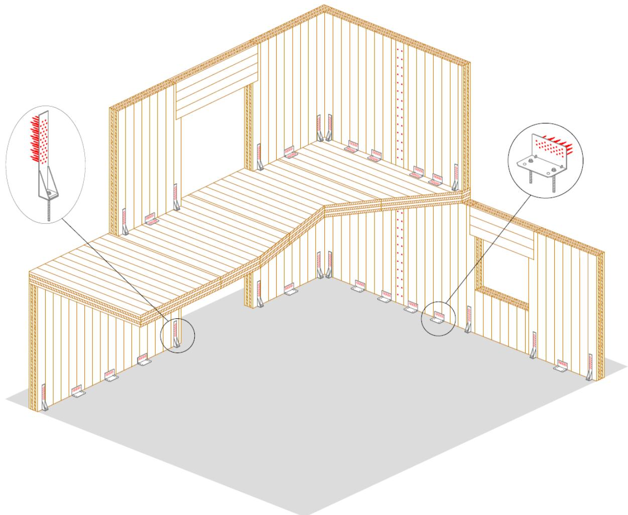
**Figure 1 - CLT building in ductility class DCM: dissipative zones**
